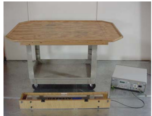
EN 61000-4-4 Electrical Fast Transients 4 kV Direct, 2 kV Injection
